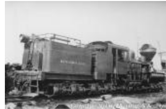
Locomotive with rear light and spark arrester (2020_06_08_06_004)
